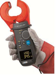
**New safety feature: the ground voltage function!** If the voltage present exceeds the safety voltage threshold, the "dangerous voltage" symbol flashes on the screen and the buzzer sounds an alert signal.
