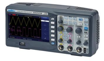
The display allows you to view 32 measurements at the same time as the measurement dashboard.
