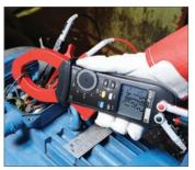
Network quality analysers: determine the total harmonic distortion. These instruments decompose the voltage and current signals and then calculate the RMS value of each frequency in the signal. A Qualistar will also indicate the total distorting current (or voltage) to allow correct sizing of an anti-harmonic filter.
