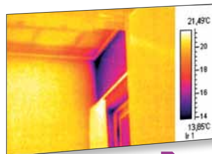
Heat losses as seen from inside a room. As defined by the scale, you can see all the areas where cold air enters, coloured black and mauve.
