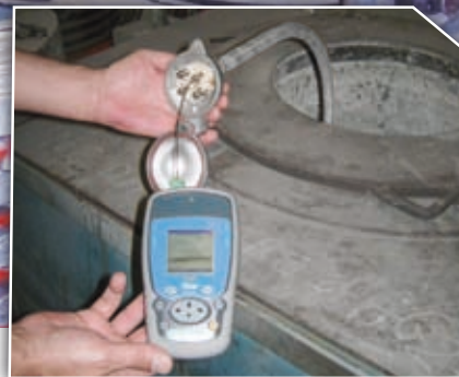
Elbowed temperature sensor assembly for aluminium foundries.
