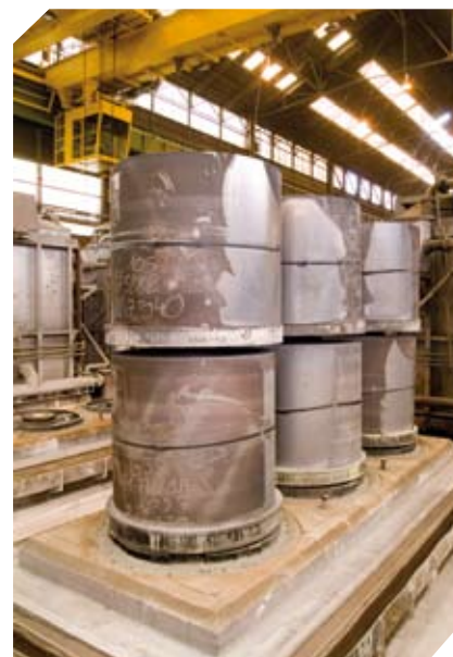
➔ View of a removable-cover furnace base with its 6 rolls of steel after heat treatment.
