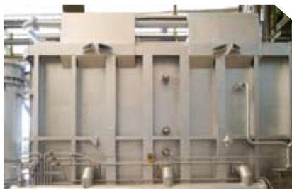
New removable-cover furnace during installation of instrumentation.
