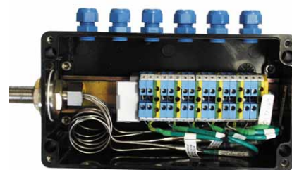
Authorised multipoint pyrometer casing Intrinsic safety
