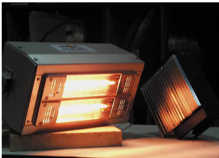
The infrared lamps used for drying paints require very constant heating power control.
